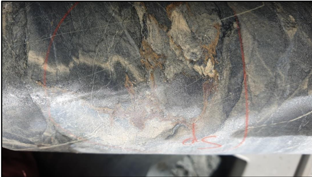
Figure 3: Example of quartz-carbonate veining in hole OKDD001, 53.1m
