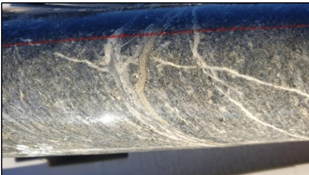
Figure 4: Example of multi-phase quartz-carbonate veining in drillhole OKDD001, 257.4m
