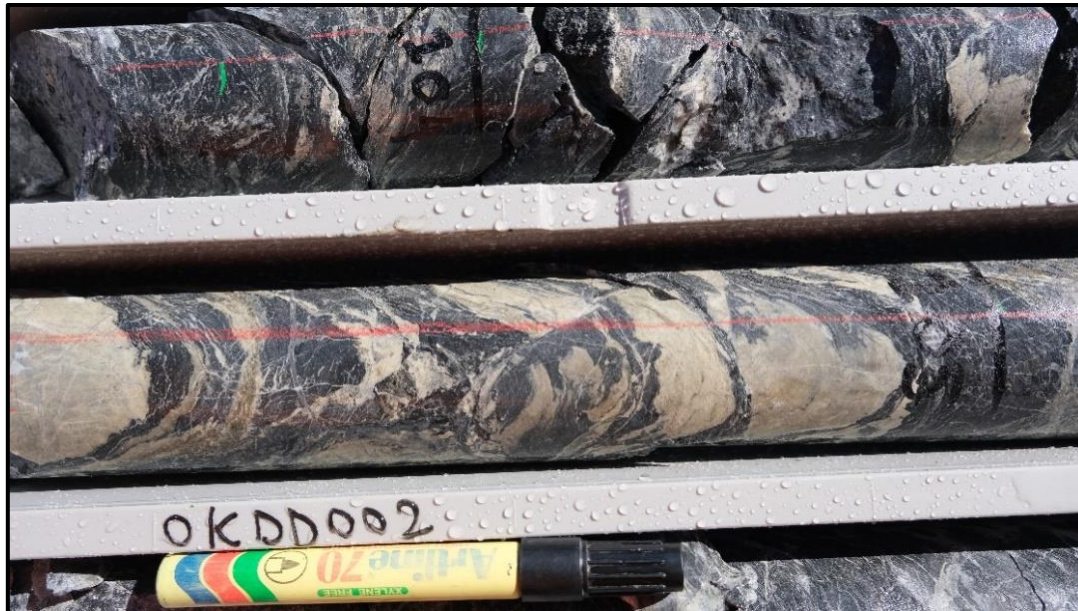
Figure 5: Example of mylonitic zone comprising altered granitic material and black sediments with quartz-carbonate veining in drillhole OKDD002, 104.8m
